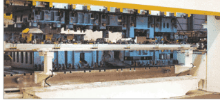
2000ton Transfer Press with Blank Carrier
